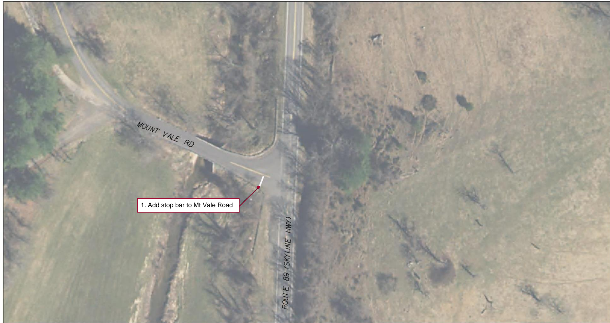
Figure 5 – Near-Term Intersection Improvements
