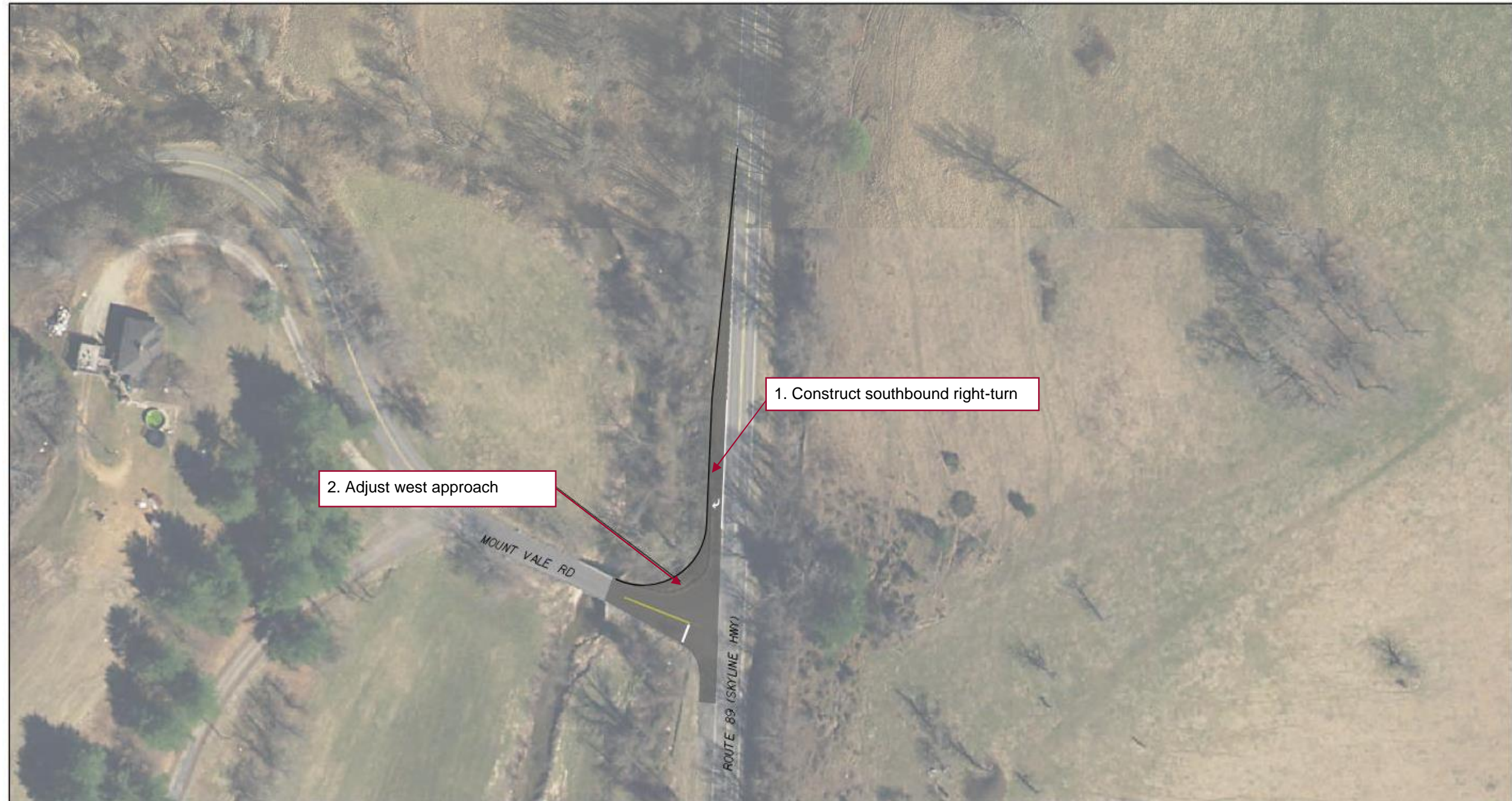
Figure 6 – Intermediate-Term Intersection Improvements
