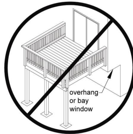
Figure 18. No Attachment to House Overhang with Ledger.
